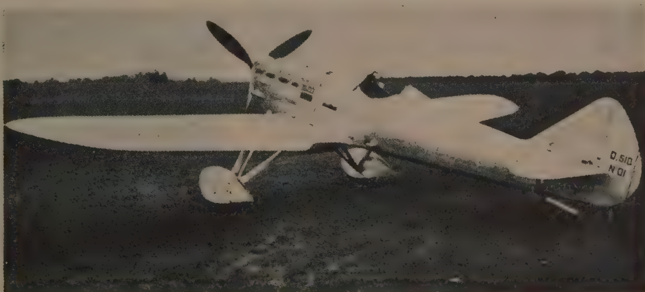
French Dewoitine D. 510, a single-seat fighter equipped with an Hispano- Suiza 12 Yvrs motor- cannon.
